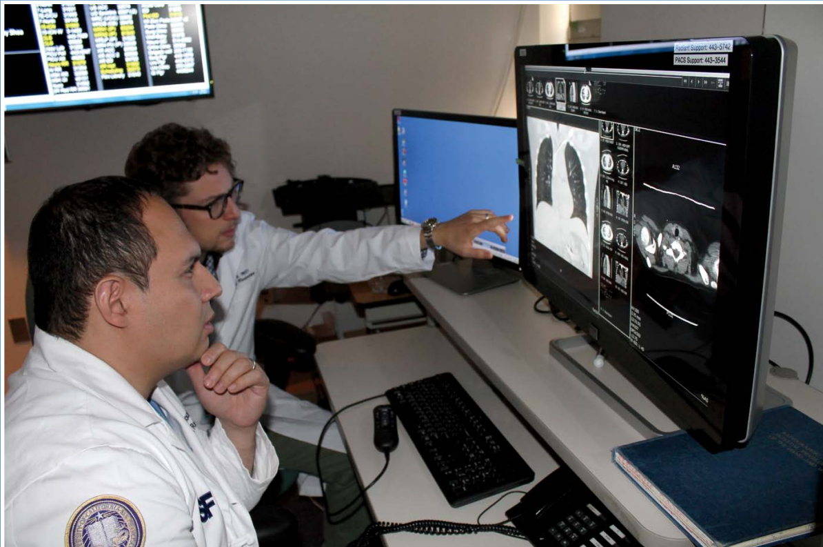
Our latest configuration, seen in the Pediatric Radiology reading room: a 6Mpixel single monitor with adjacent text monitor.
