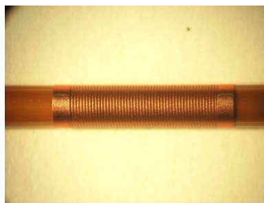
Figure 2: 50-turn helical coil patterned on a 1.37 mm OD polyimide cylinder. 0.5 mm collars at each end are solder attachment pads.
