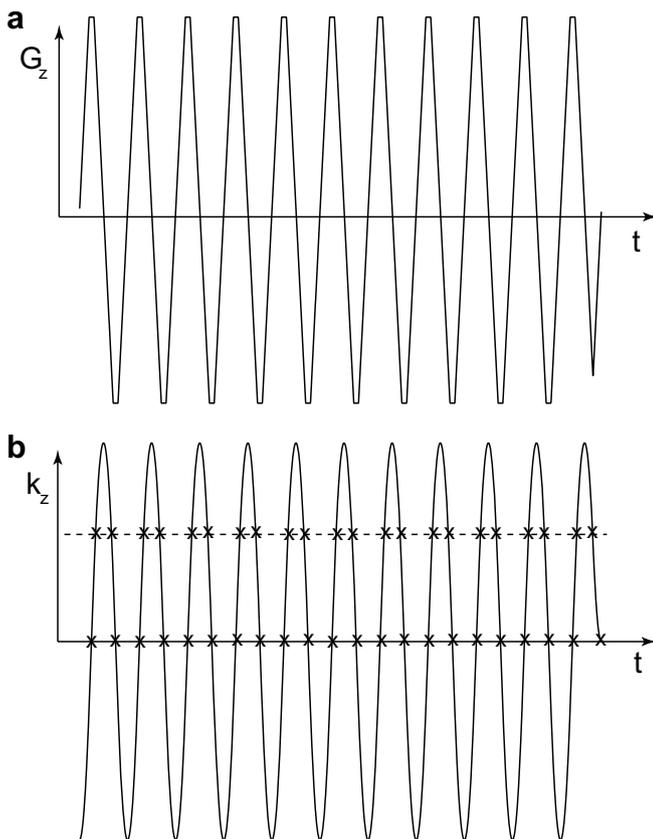
**Fig. 1.** The zig-zag trajectory through excitation  $k$ -space. (a) A gradient waveform used with a typical spectral-spatial RF pulse. (b) The integral of the gradient shape gives the trajectory through excitation  $k$ -space. The “x” marks show that the sample spacing across the central region is uniform, but is staggered away from the center. Compensating for this staggered sampling is the key to the design technique used in this paper.
