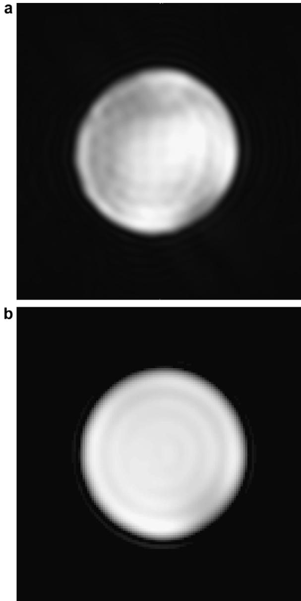
**Fig. 5.** Phantom experiment showing spatial resolution of the new pulse sequence. (a) New pulse sequence, TR = 55 ms, TE = 22.5 ms, scan time = 3.5 s,  $32 \times 32 \times 16$  voxels. (b) Conventional chemical shift imaging (CSI) sequence with phase encoding in both in-plane directions, TR = 600 ms, TE = 1 ms, scan time = 614 s,  $32 \times 32 \times 1$  voxels. For both scans, the FOV was 8 cm and the slice thickness was 5 mm.
