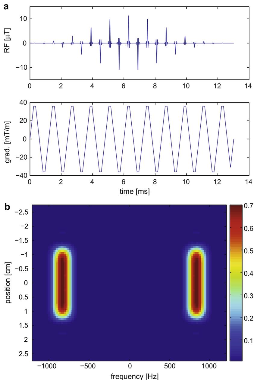
**Fig. 2.** Spectral-spatial RF pulse designed for imaging single components of the  $^{13}\text{C}$  spectrum. (a) The RF pulse and gradient waveform. (b) The excitation profile of the spectral-spatial pulse as a function of frequency and position, with the color corresponding to the magnitude of the resulting transverse magnetization normalized by  $M_0$ . Note the large spectral stopband and the sharp spatial selectivity of the pulse.
