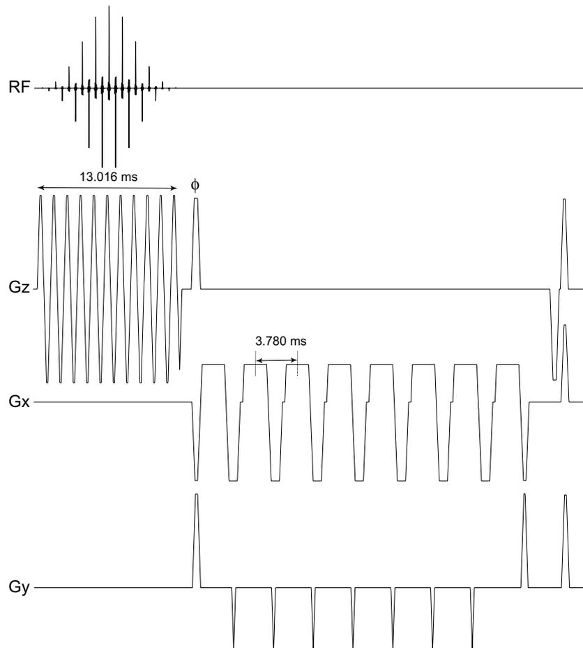
**Fig. 4.** Echo-planar pulse sequence used in experiments. The sequence consists of a 13.016 ms spectral-spatial RF excitation pulse followed by a gradient lobe to phase-encode the through-slice direction (labeled  $\phi$ ). The four lobes of the echo-planar readout gradient on  $G_x$  are separated by 3.780 ms, with blips on  $G_y$  in between.
