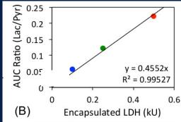
Phantom layout with varying concentrations o enzyme, B) Measurement of hyperpolarized signa in LDH trapped alginate microspheres with 0.1 (blue), 0.25 (green) and 0.5 (red) kUnits.
